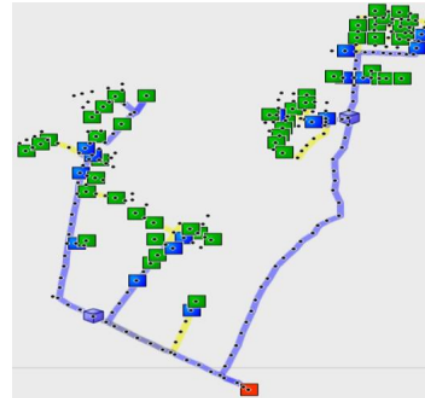
Figure 10. Branching Method Cable Route
