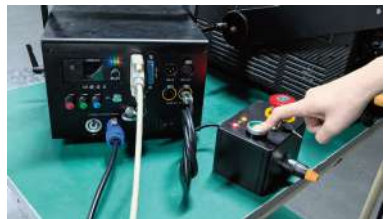
F: Press down the START button on the E-stop box. Turn the keys and the power switch at the back of the laser system to the ON positions.
